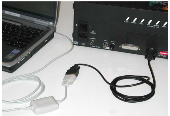
The Iotech ChartScan™ data recorder connected to a laptop PC using a USB to RS-232 converter
